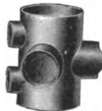
MAKING CRESCENT CRANK HANGER. STAGE 4.
