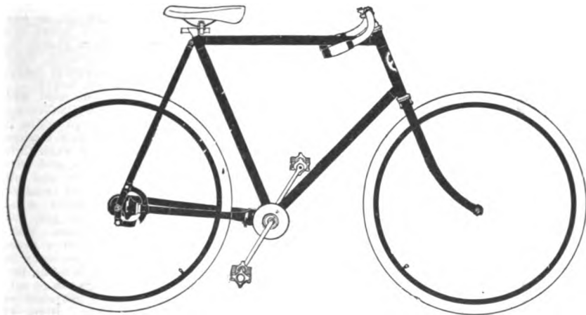
CHAINLESS TYPE, 1898 (BEVEL GEAR).
