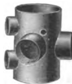
MAKING CRESCENT CRANK HANGER. STAGE 5.
