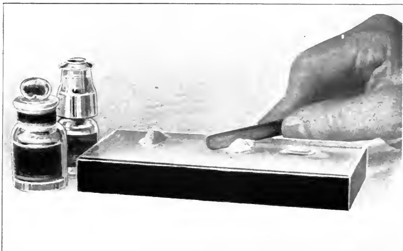
Fig. 95.—Taking the first portion of the powder which should be about half of the entire amount needed.
