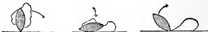
Fig. 100.—Illustrating in three successive steps the method of removing the mix from the spatula to the slab.
