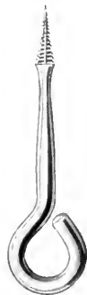
Fig. 30.—Short-Shank Screw-Porte. Without handle. The shank has a ring end for receiving a small bar as a handle.
