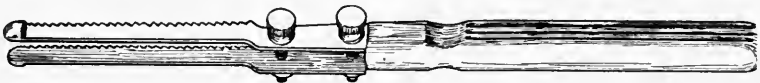
Fig. 246. Adjustable double-bladed saw, which is very useful when the case permits of making parallel cuts through the bone.
