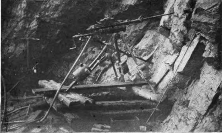
FIG. 53.—Ingersoll-Rand 3½" Piston Drill
