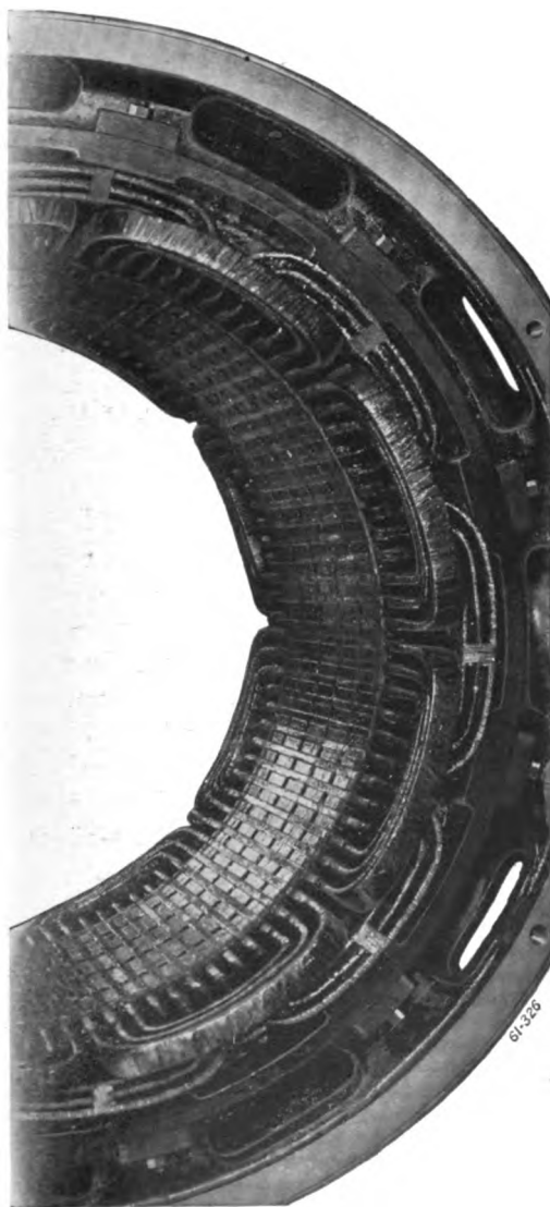
FIG. 315. A three-phase armature winding having three slots per phase per pole. Wagner Electric Co.
