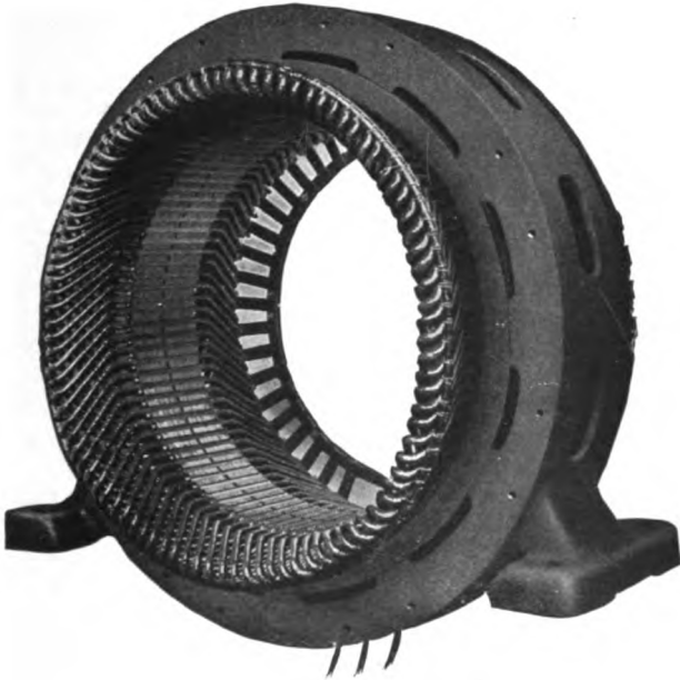
FIG. 353. A stator wound like the rotor in Fig. 352a. It has a full pitch winding, with a coil pitch of eight. Westinghouse Electric & Mfg. Co.
