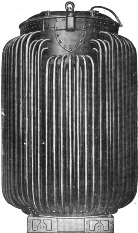
FIG. 79. Additional cooling surface is furnished by the pipes. The oil which carries the heat from the core and coils circulates through the pipes and is cooled. General Electric Co.
