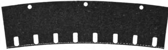
FIG. 156.—CORE-SEGMENT OF 64-POLE ALTERNATOR (HEYLAND).
