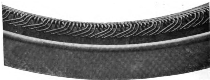
FIG. 290.—WINDING OF LAHMEYER ARMATURE (THREE PHASE), 300 KW, 64 POLES, 94 RPM, 240 VOLTS.
