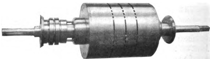
FIG. 357.—ROTATING FIELD-MAGNET, 2-POLE, 400 KW (BRITISH WESTINGHOUSE CO.).
