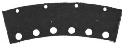
FIG. 160.—CORE-SEGMENT OF THREE-PHASE ALTERNATOR AT PADERNO.
