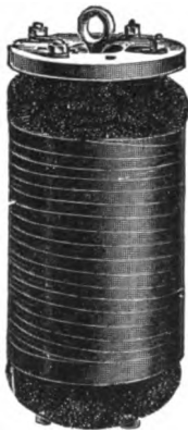
FIG. 410.—SWINBURNE'S HEDGEHOG TRANSFORMER.
