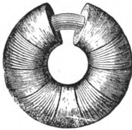
FIG. 394.—RING TRANSFORMER, WITH SANDWICHED COILS.
