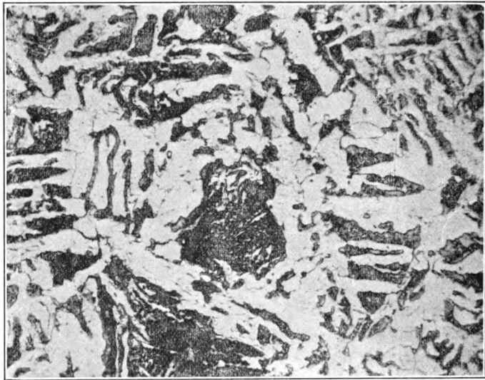
FIG. 158—Typical Structure of Plate Just Below Weld, Etched with Nitric Acid and Magnified 400 Diameters
