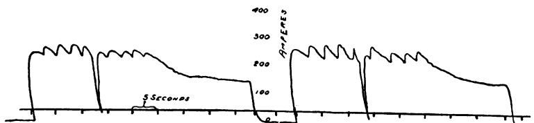
-Current curve taken by graphic recording ammeter on a car equipped with multiple unit control with automatic accelerating device.
