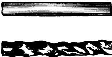
Fig. 11. Tantalum Filament Before and After 1,000 Hours' Use.
