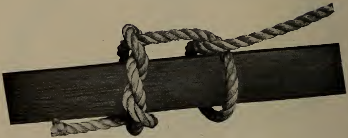
Fig. 30 TIMBER AND HALF HITCH
