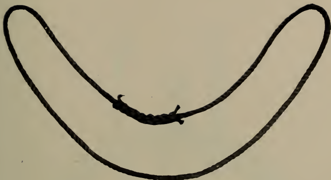
Fig. 31 SPLICED ROPE SLING
