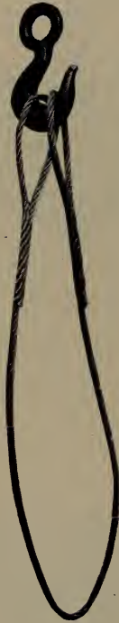
Fig. 33 WIRE CABLE SLING
