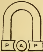
Fig. 51.—Permanent Magnet with Iron Pole Pieces (P) and Armature (A).
