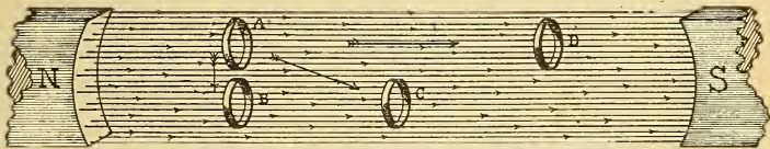
Fig. 273.—No Induced Current in a Loop When Moved so That There is No Rate of Change of the Magnetic Lines Through It.
