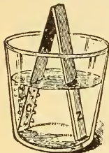
Fig. 69.—Copper and Zinc in Acidulated Water.
