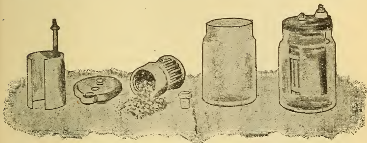
Fig. 89.—Elements of Carbon Cylinder Cell with Depolarizer.
