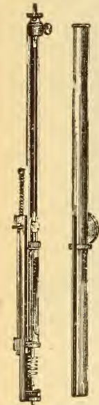
Fig. 171.—Details of Removable Suspension Coil and Tube.
