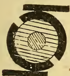
Fig. 315.—Section of Two-Part Commutator.
