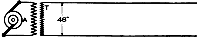
FIG. 1030.—Required, the size of wire to deliver 5,000 K.W., 20 miles with 10% line loss; power factor 85%, frequency 60 cycles, nominal voltage of transmission 33,000; spacing between wires 48".
