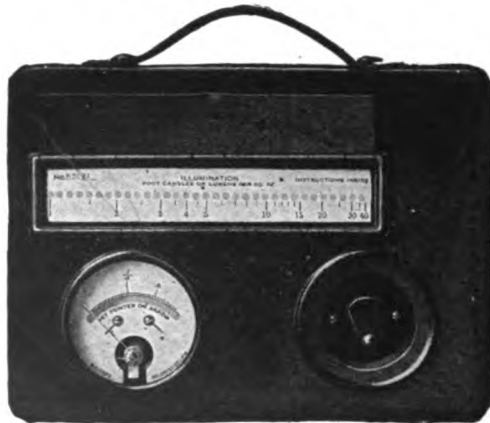
FIG. 1270.—Exterior appearance of foot-candle meter, built by the General Electric Company.
