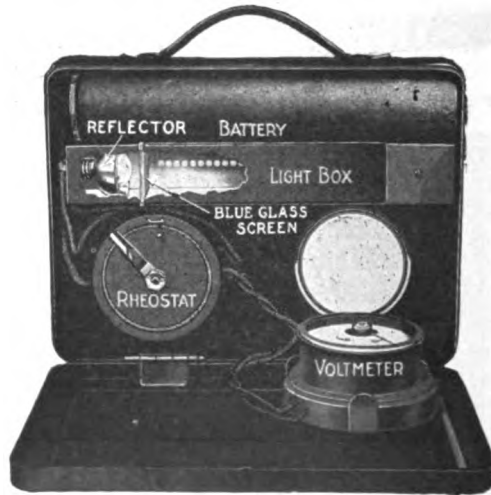
FIG. 1273.—Interior details of foot-candle meter.
