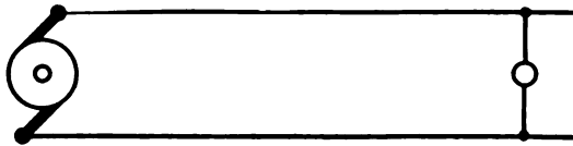
FIG. 1028.—Required, the size of wire to deliver 500 40-watt, 110-volt lamps, 400 feet, 120 volts at generator.
