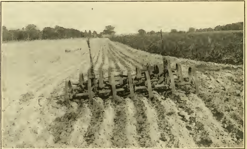
FIG. 12.—A spring-tooth harrow, showing its use in preparing sandy-loam land, after plowing, for corn.
