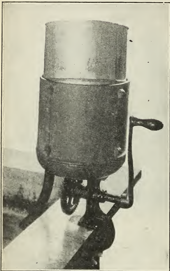
FIG. 9.—Small hand-power vegetable peeler. The potatoes are thrown by centrifugal motion against the carborundum lining, which nicks off the skin in small bits. Fresh water drips through the perforated pan at the top, carrying away the skins through the rubber waste pipe at the base.
