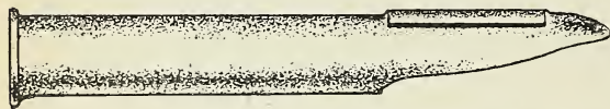
FIG. 3.—Small apple corer or vegetable peeling knife used to remove eyes and diseased spots from potatoes. There is a blade at the side, and if a mechanical peeler is not available knives of this description are better for peeling than ordinary paring knives.
