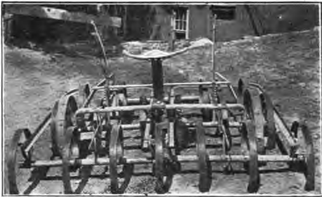
FIG. 7—A USEFUL TYPE OF SPRING-TOOTHED HARROW
