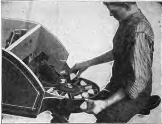
FIG. 29—THE PLATFORM OF THE ROBBINS IMPROVED PLANTER
