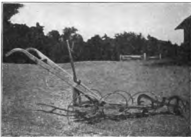
FIG. 33—ONE-HORSE SPRING-TOOTH CULTIVATOR
