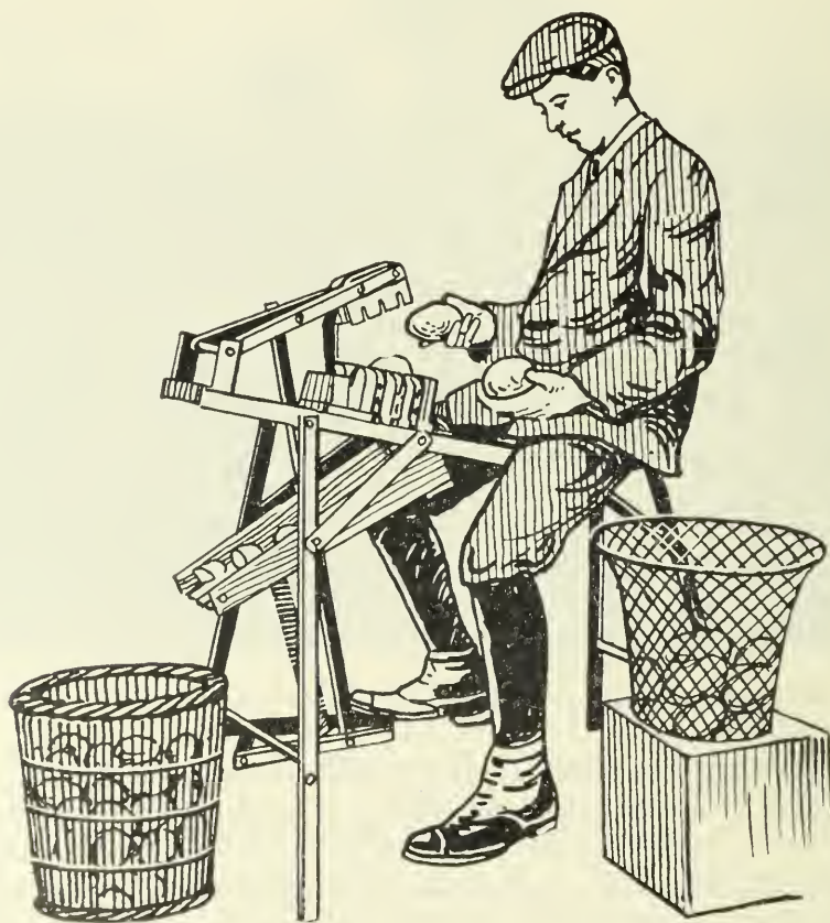
Cutting seed pieces by foot power machine.
