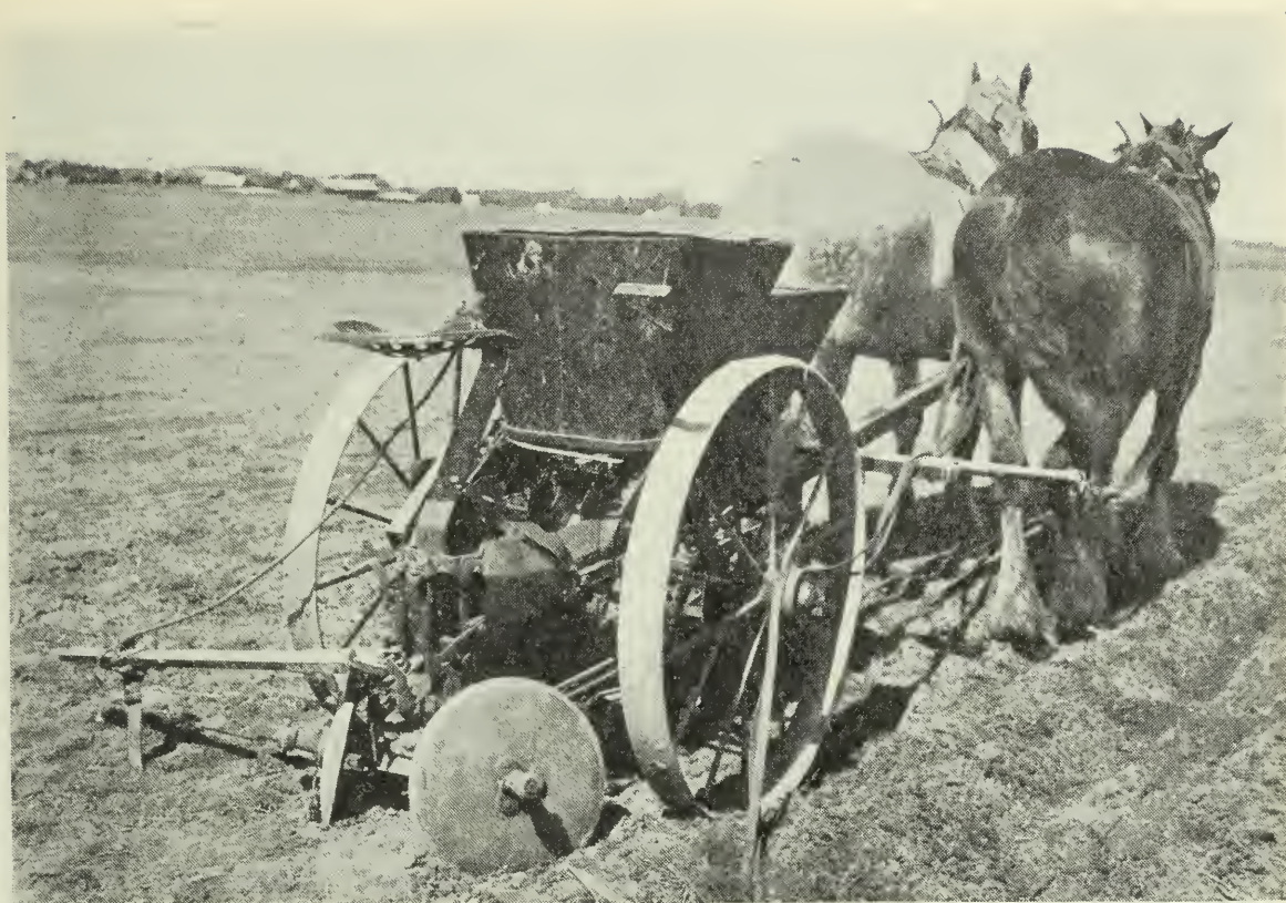
A combined planter and fertilizer drill, single row picker type.
