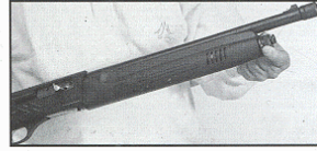
Fig 5A: Screw on the forend cap so that the forend is held firmly in place. With the forend in place and the barrel in place and the forend cap securely in place, depress the carrier
