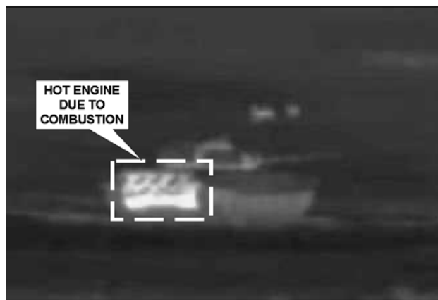
Figure E-3. Heat caused by combustion.
