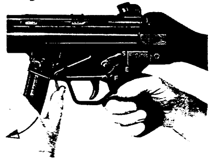
Ill.# 23B - Removing the magazine
