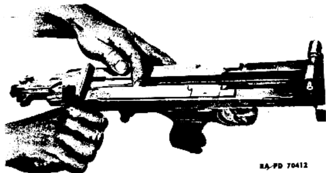
Figure 49 - Removal of Bolt
