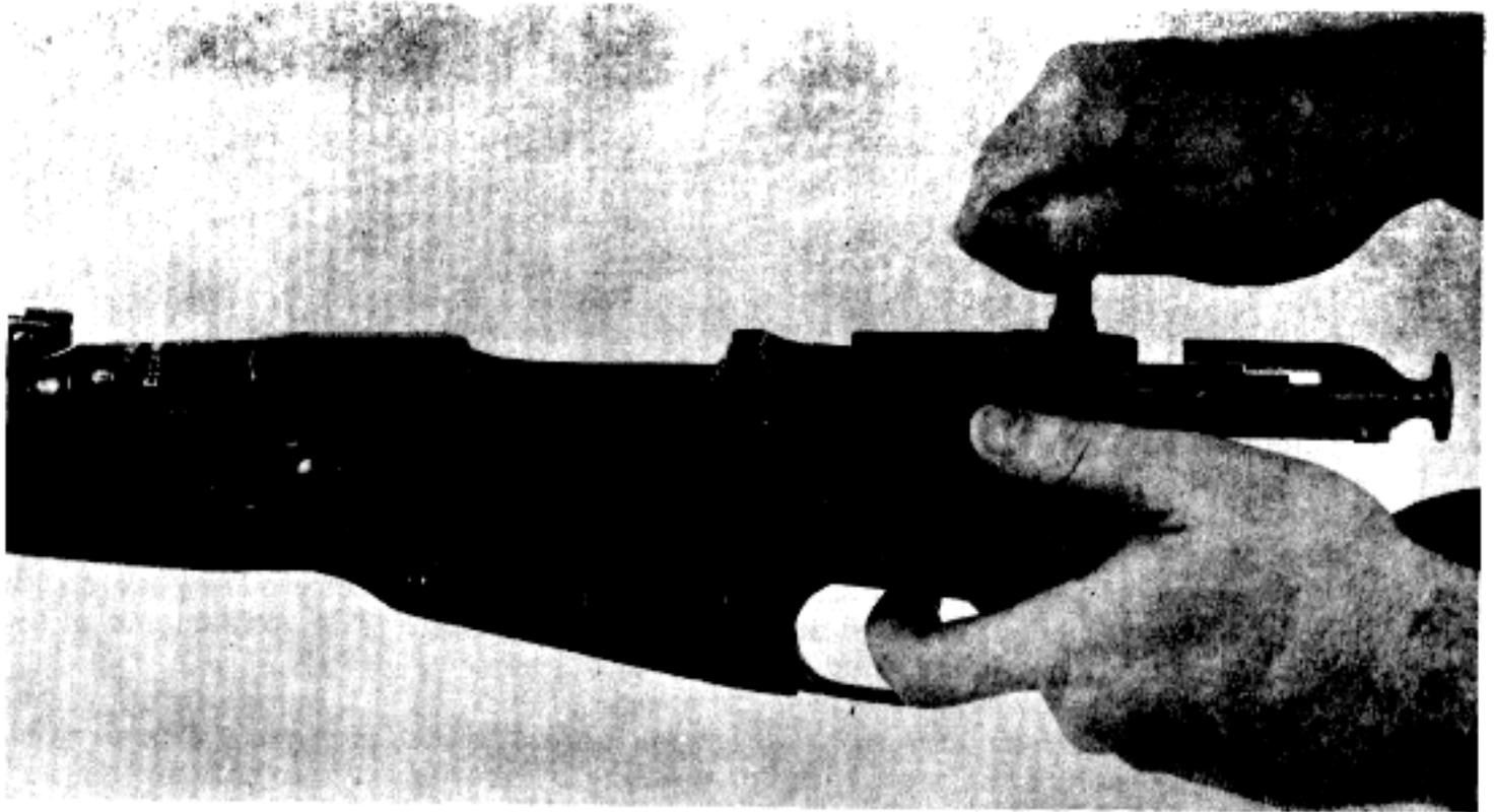
FIGURE 45. REMOVING THE BOLT.
