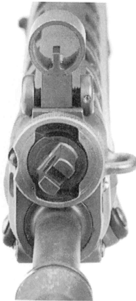
Gas valve in position II
