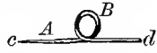
Fig. 77.—A, body of pin; B, loop made in middle of pin; c and d, ends of pin.
