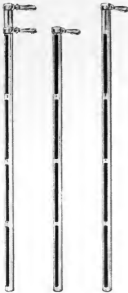
FIG. 53. The McKay sampler.
