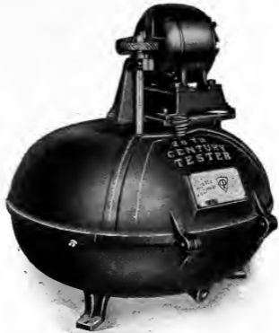
FIG. 25. Type of Babcock electrical testers.
