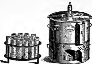
FIG. 47: The Gerber fermentation test.
