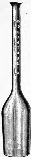
FIG. 5. Babcock milk test bottle.
