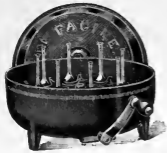
FIG. 20. Type of Babcock hand testers.
