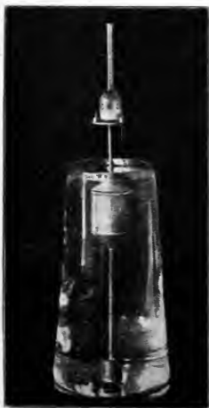
FIG. 35a. The Wisconsin hydrostatic cream balance.
