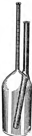
FIG. 37. The double-necked skim milk bottle (sometimes called the Ohlson or B. & W. bottle).
