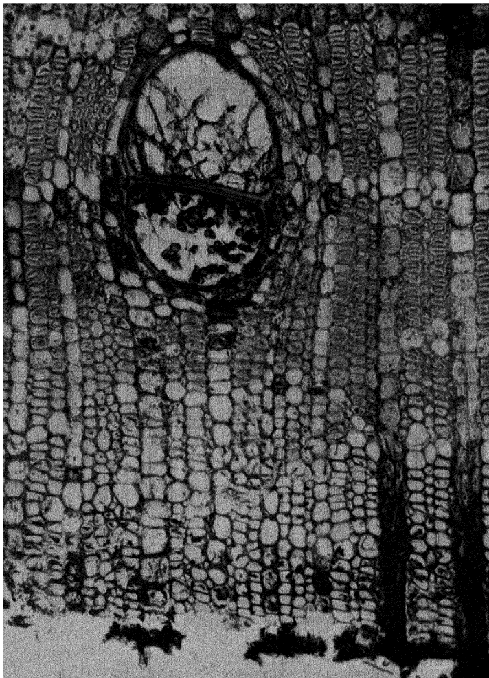
FIG. 30.—Mouldy rot. Section through outer infected area, showing the macrospores developing in the outermost wood vessels. \times 333 .
