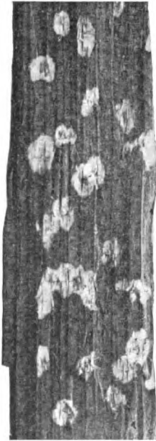
FIG. 23. — Pecky wood-rot; early stage in Douglas fir.
