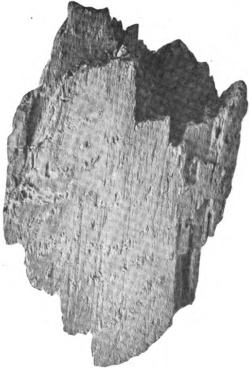
FIG. 12. — Beech wood decayed by Fomes applanatus .
