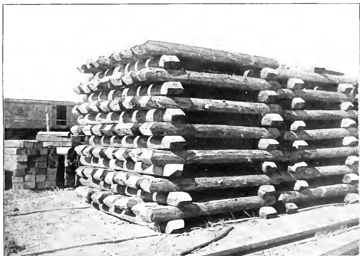
FIG. 2.—AFTER TREATMENT. LOGS POLE PINE, OPEN-CRIB PILE.
