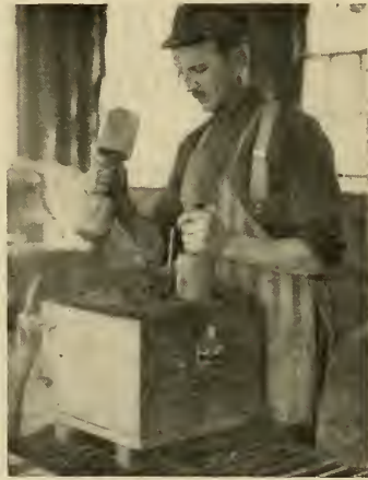
FIG. 4.—BUTT-RAMMING THE SURFACE OF THE MOLD.
