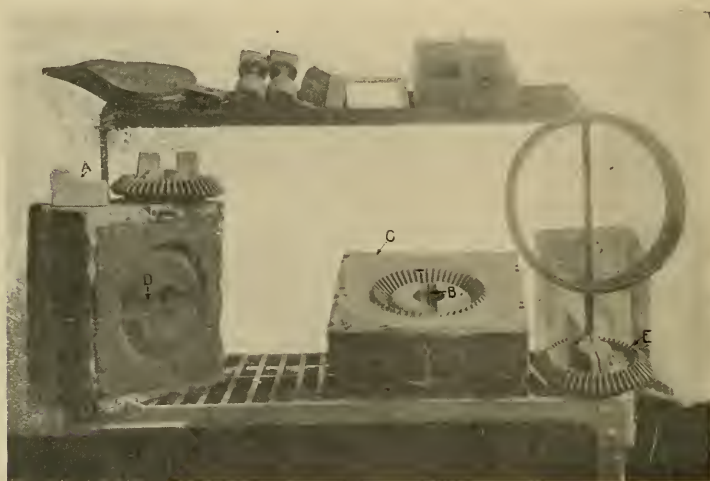
FIG. 16.—MOLDING AND SPLITTING A BEVEL GEAR.
