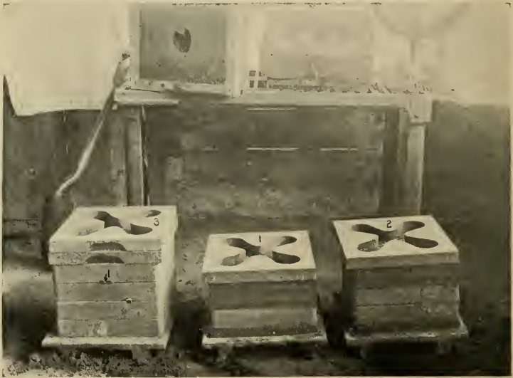
FIG. 5.—MOLDS WEIGHTED FOR POURING.
