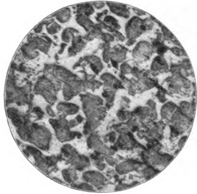
FIG. 2. WHITE CAST IRON POLISHED IN RELIEF. MAGNIFIED 100 DIAMETERS.
