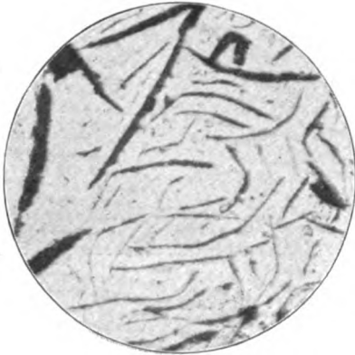
FIG. 1. GRAY CAST IRON POLISHED BUT NOT ETCHED. MAGNIFIED 56 DIAMETERS.
