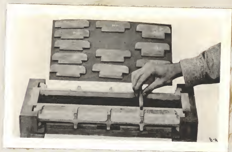
Fig. 5. Use of Strikes to Level Sand in Mold Box for Doty Test.
