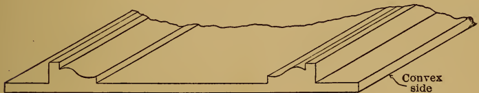
FIG. 7.—Thin Flat Plates, Unequal Shrinkage.
