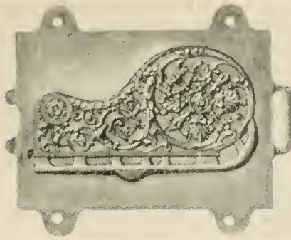
Fig. 34—Match-plate for a brass, cash register casting
