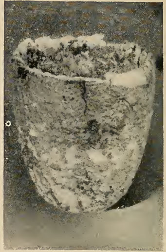
Fig. 37—Crucible showing the cracks which begin to form at the top when its life is nearly ended
