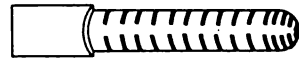
FIG. 101.—Neumann bands revealed as continuous strata by etching a cylinder turned from a meteorite. Stead.
