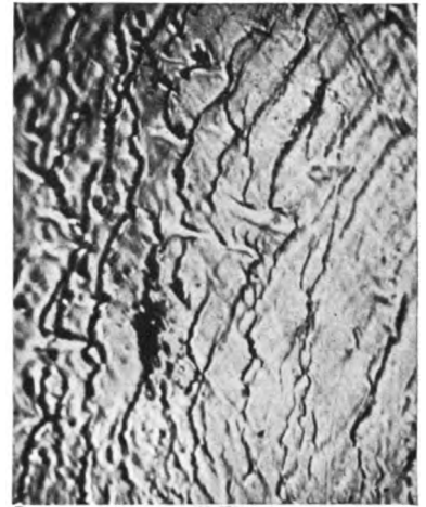
C. Irregular slip-bands in ferrite. \times 500
