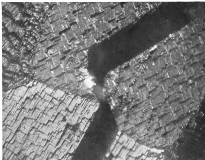
E. × 50 Rectangular etching figures and rupture in silicon steel.—STEAD. §738.
