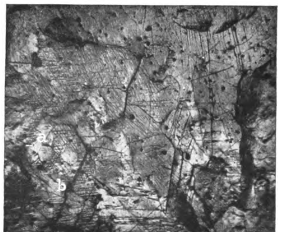
F. Grain-uplift and slip-bands in austenite. §409, 412. × 50
