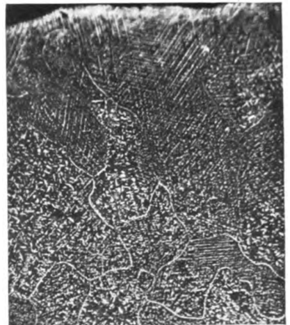
F. Pro-eutectoid cementite assembled in grain boundaries and octahedral planes. Manganese steel. §388, 405. \times 50
