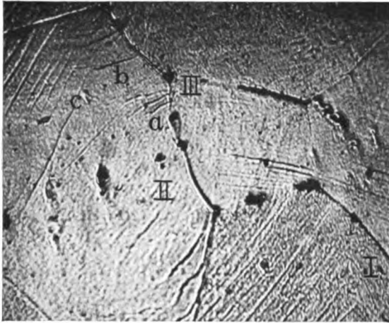
A. Slip-bands in etched ferrite. × 500
