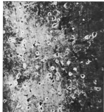
D. Ferrite rings about graphite centers in 1.45 carbon steel. §289. × 42
