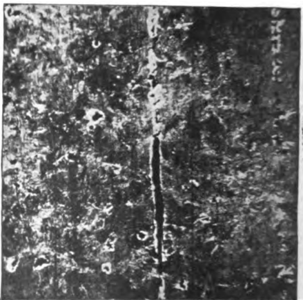
G. Ferrite rims about graphite ghost lines in 1.45 carbon steel. §§108, 289. × 42
