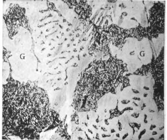
A. X 47 White cast-iron, the chilled face of tread of wheel. §§304.
