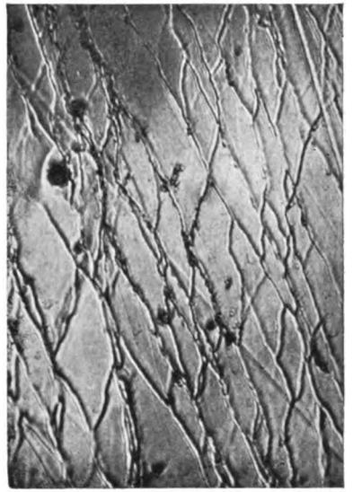
E. Irregular slip-bands in ferrite. \times 500
