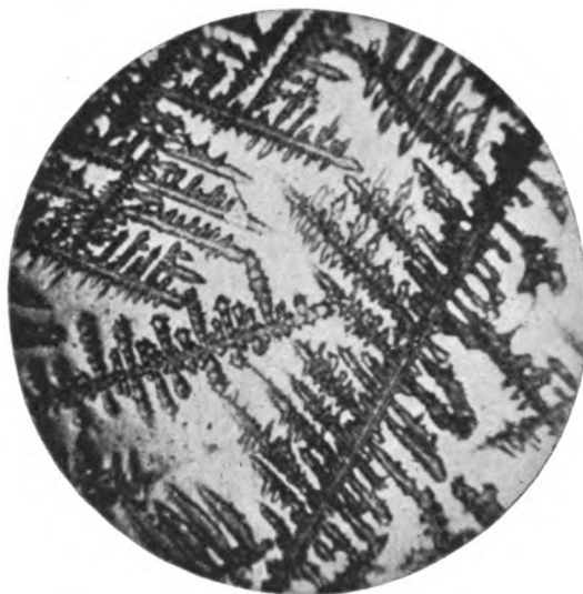
FIG. 108.—Interlacing of pine tree branches from adjoining grains in sal ammoniac, causing a boundary region of mixed orientation. Rosenhain. 2
