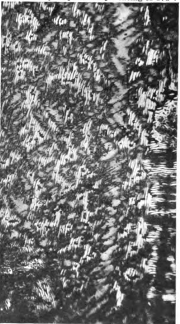
G. Eutectiform pattern related to dendrites.
