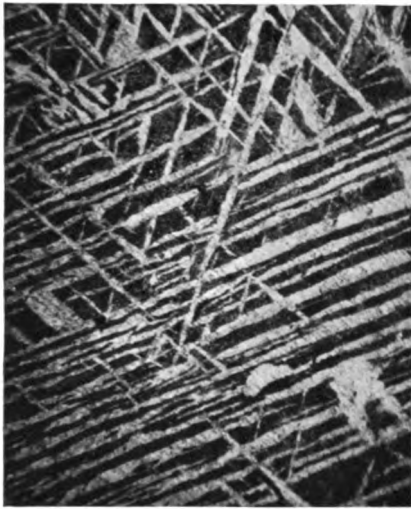
A. Widmanstätten structure of ferrite. C=0.40. × 50
