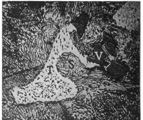
F. X 500 Eutectic, T, pearlite, S, and slag, V.
