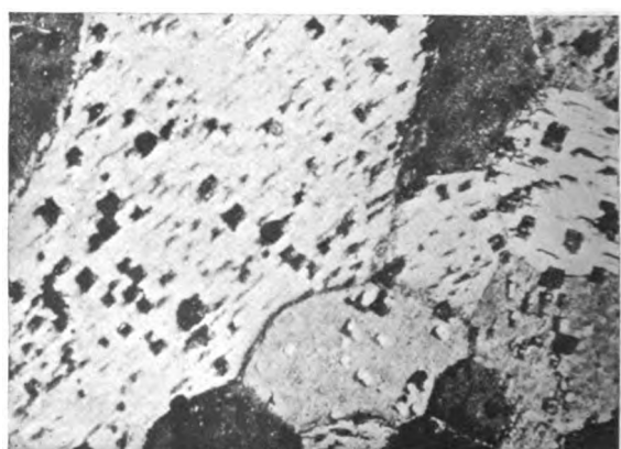
H. \times 60 Cubic etching pits in silicon steel.—Stead. §371.
