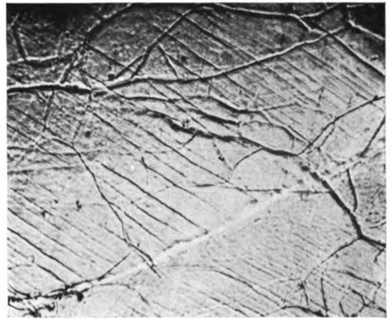
B. Slip-bands crossing grain boundaries in pre-etched ferrite. §425. × 500
