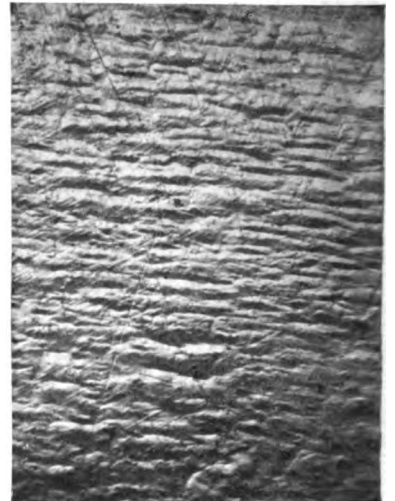
B. \times 50 Surface crumplings in manganese steel. §411.
