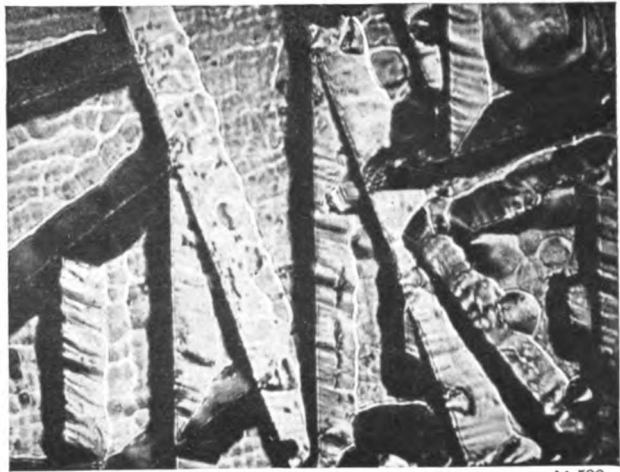
F. 6 directions of Neumanns on cube face. Detail of Fig. A. §602. \times 500
