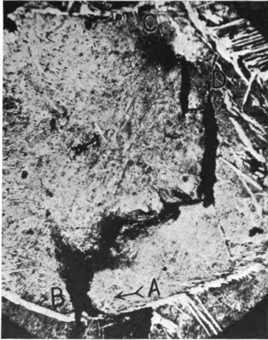
C. Rupture escapes ferrite network. C=0.59. §§717, 725.
