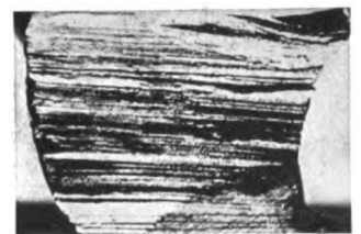
G. \times 1.4 Fibrous fracture in nickel. §762.
