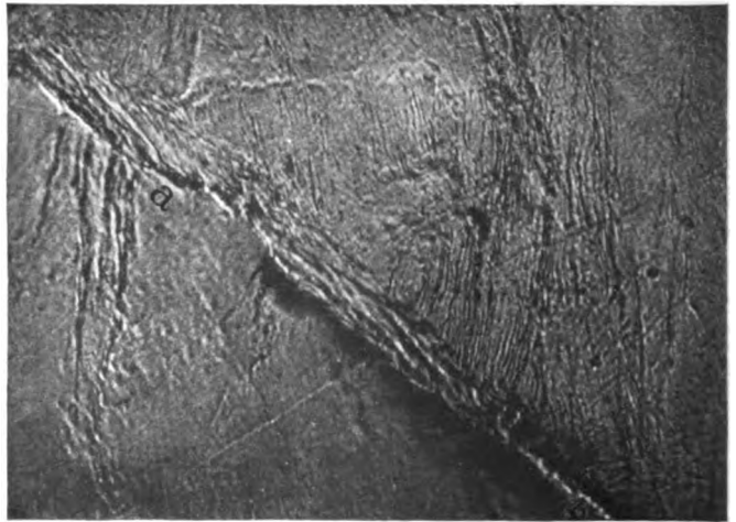
F. Extrusion of ferrite network ab and of pearlitic ferrite in steel of 0.59 C by pressure. Same as Fig. E. §§531, 543, 725. × 500
