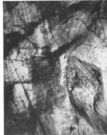
G. Slip-bands cross dendrites and grain boundaries. \times 50
