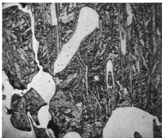
B. 765°. Cementite + martensite + pro-eutectoid cementite needles.
