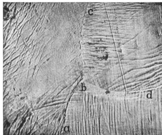
F. Slip-bands in ferrite. §§408, 412. \times 500
