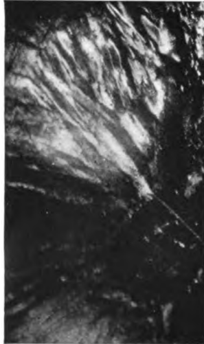
AA. \times 6 Persistence of columnar structure through 1100° quenching in Mn steel. §408.
