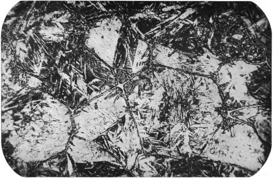
A. Quenched from slightly above solidus. Much twinning. §264.
