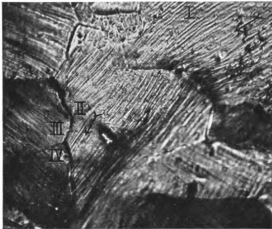
C. Slip-bands in etched ferrite. × 500
