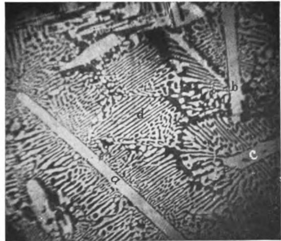
G. Hyper-eutectic cast-iron. White bands a, b, c of primary cementite; honeycomb d of eutectic. §§81, 175. \times 30
