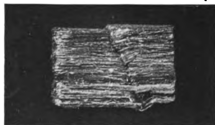
E. Lüder's lines in compressed wood. §395. \times 2.7
