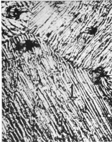
A. Etching lines without heating. \times 500
