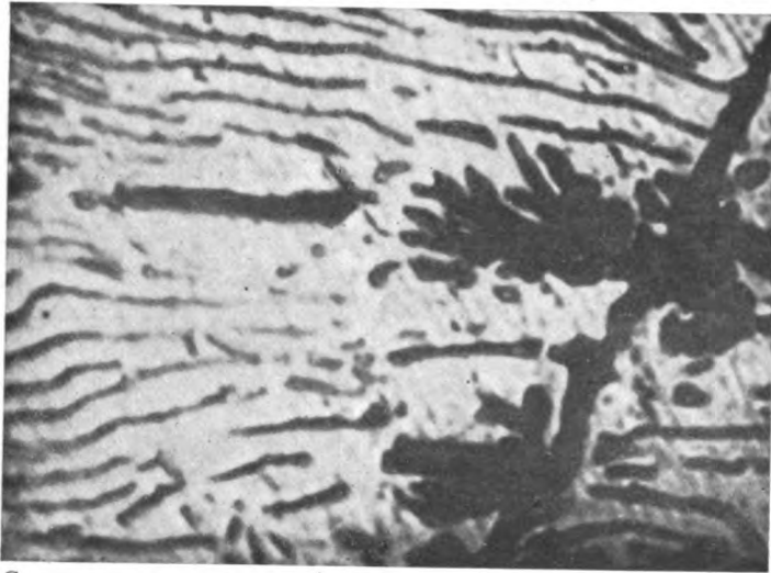
C. Hyper-eutectoid steel. Carbon 1.14. Etched with sodium picrate. \times 3300 Black = cementite, white = pearlitic ferrite. §§71, 74.
