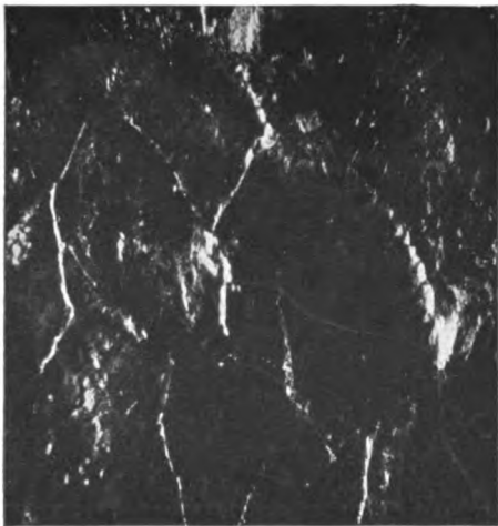
E. Extrusion of ferrite network by pressure. Oblique light. C=0.59. §§531, 725. × 50
