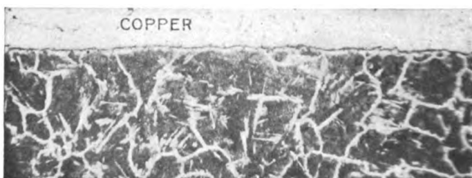
D. \times 50 Fe 3 C expelled to outer surface of steel of 1.45% carbon, then copper plated. §368.
