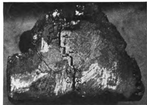
D. × 2.5 Rupture seeks grain centres in bismuth. Etched. §694.
