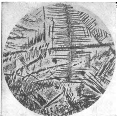
C. Dendritic structure in rolled carwheel. §§343, 762, 796. \times 1
