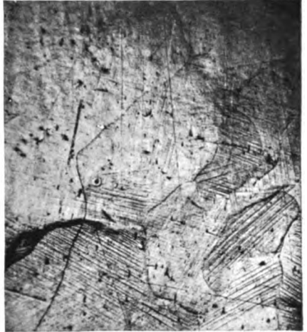
D. Expulsion of Fe_3C masks pre-existing slip-bands. §368. \times 500
