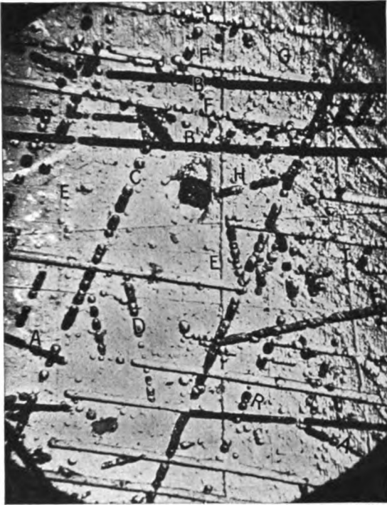
A. 8 directions for Neumanns on cube face. §590. \times 50
