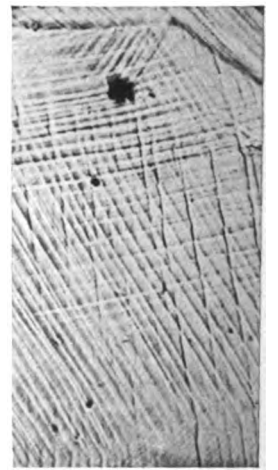
H. \times 50 Four directions of slip-bands.—Invar. §417.
