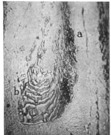
F. × 1200 Movement of pearlitic cementite sheets in punching.—Howe and Levy. §541.
