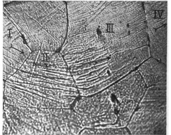
D. Slip-bands cross grain boundaries in etched ferrite. × 500
