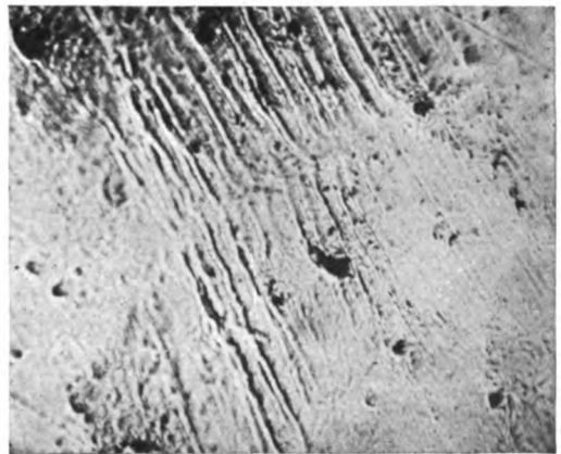
D. Slip-bands in Widmanstätten ferrite bands of Fig. A. Unetched. C=0.40. × 500
