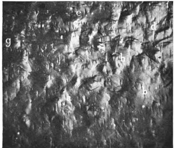
D. Grain-uplift and slip-bands in austenite. §408. × 50
