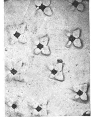
F. Pressure squares round holes.—STEAD. §379.
