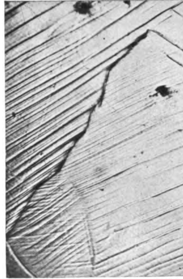
E. Slip-bands stop or change prominence at boundaries. \times 500
