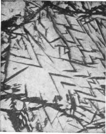
A. Martensite (black) in austenite.— STEAD. §99. \times 100
