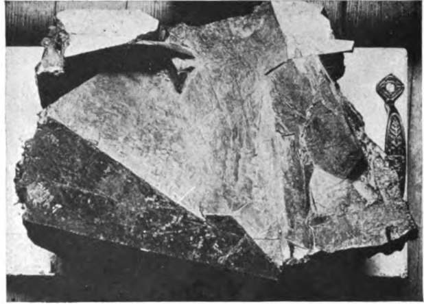
B. × 0.22 Cementite plates in fracture of spiegeleisen. §731.
