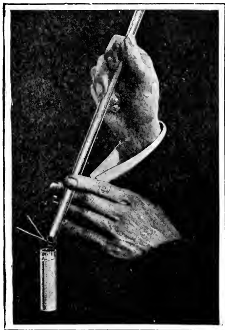
Fig. 166—Inserting the tube in the mercury receptacle
