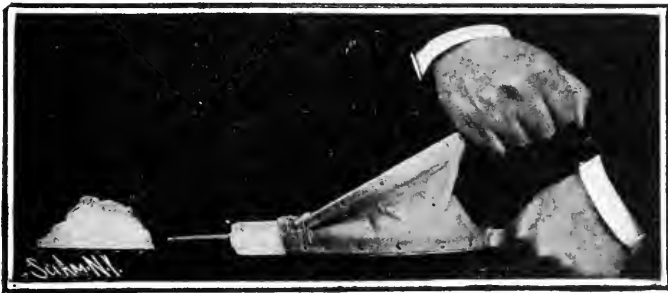
Fig. 183--Making frost with carbon disulphide
