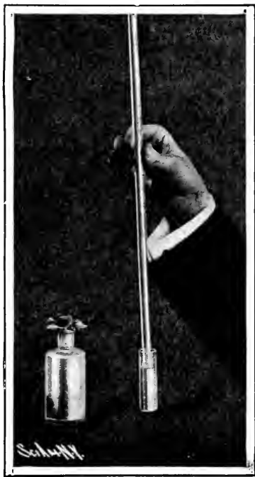
Fig. 167—The tube immersed in the mercury receptacle
