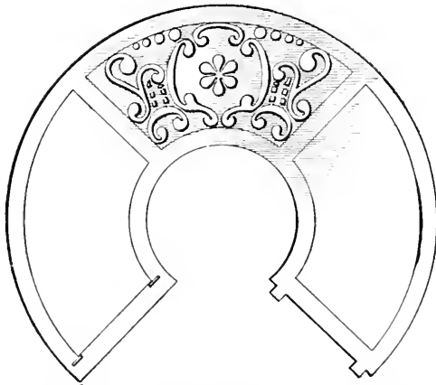
Fig. 262—A lamp-shade of brass cut with acid
