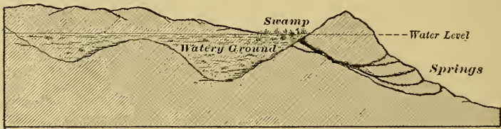
DIAGRAM SHOWING THE FLOW OF PERCOLATING WATERS
