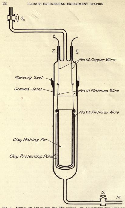
FIG. 7. DETAIL OF APPARATUS FOR MEASURING AND ANALYSING THE DISSOLVED GASES IN GLASS
