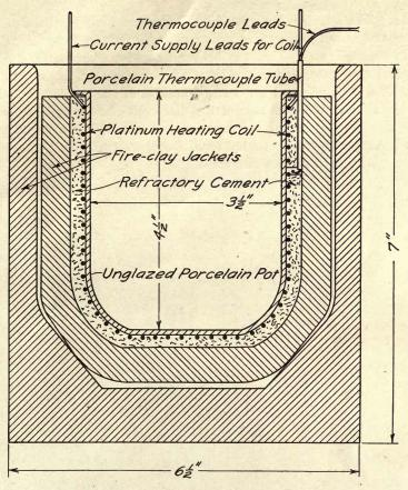
FIG. 3. DETAIL OF POT, RESISTOR, AND INSULATION
