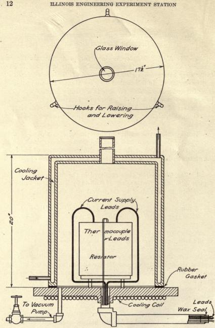
FIG. 2. DETAIL OF VACUUM FURNACE
