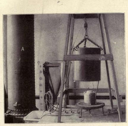
FIG. 4. VACUUM FURNACE AND LARGE VACUUM TANK
