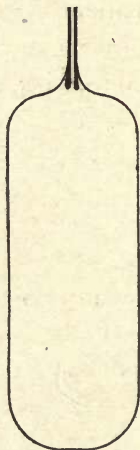
FIG. 13.—Later stage in sheet glass blowing.
