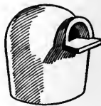
FIG. 3.—Covered pot for glass-melting, as used for flint glass and optical glass.
