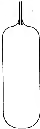
FIG. 15.—Later stage in sheet-glass blowing.
