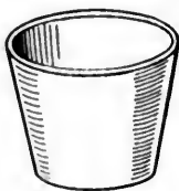
FIG. 2.—Open "pot" or crucible for glass-melting.
