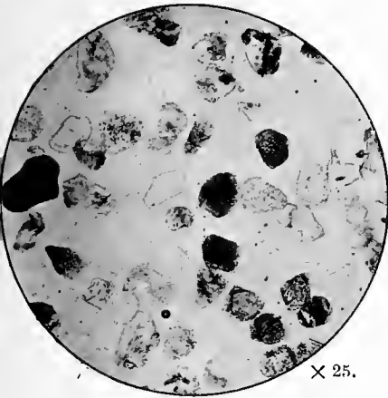
Fig. 1.—Quartz (faint and clear) and feldspar (turbid) in a good glass-sand.
