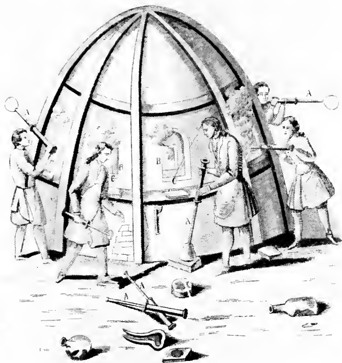
A—Blowpipes B—Glass Pots C—Working Holes Figure 12. Ancient Venetian Glass Furnace
