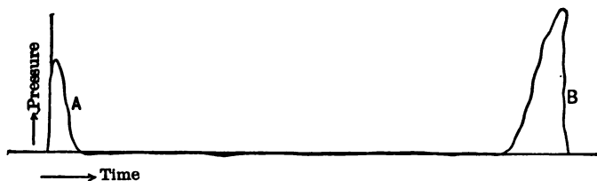
FIG. 32. Blochmann's Diagram showing Action of Subaqueous Explosions.
