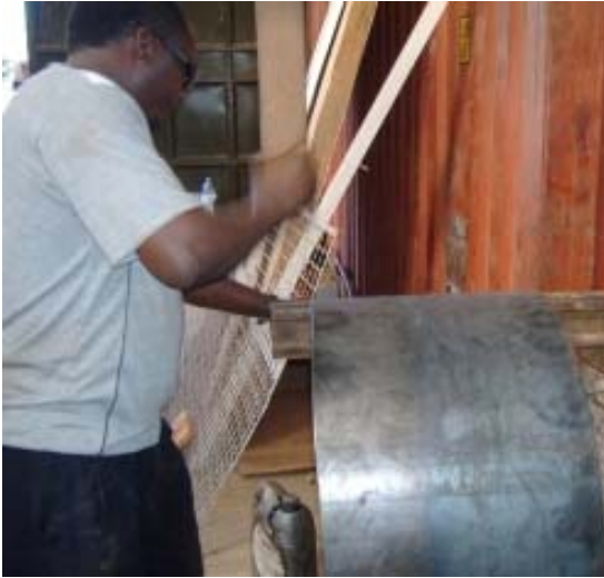
Photo 22: Metal rolling with simple hand tools
