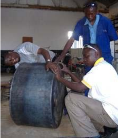
Photo 27: Welding the outer cylinder onto the base plate
