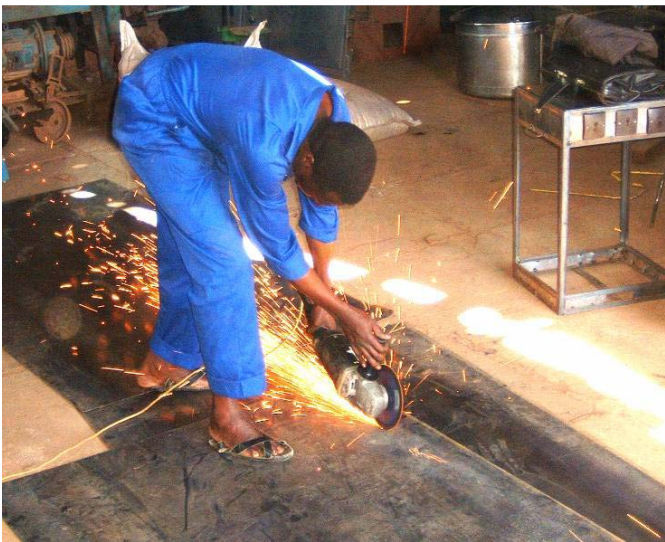
Photo 20: Metal cutting with an Angle grinder
