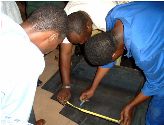
Photo 25: Marking off dimensions for the combustion chamber
