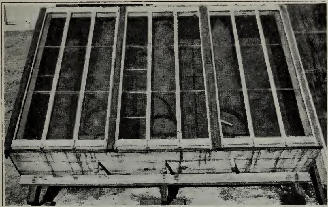
Fig. 7.—Triple-tank absorber in insulated box with hotbed sash cover.
