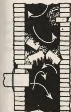
Fig. 4—This is often the bottom of the chimney in the base-cause of a poor draft. Before you use this method be sure to remove all pieces of stove pipe which extend into the chimney and which might be broken if they are left in place.
