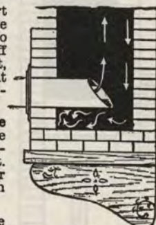
Fig. 10—If the chimney ends a short distance below the stove pipe, make a toothpick joint
