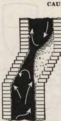
Fig. 5—Soot deposits may in time stop the draft
