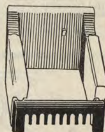
Cut Showing Arrangement of Waterbacks, Brick and Front Grates in Fire Box of Range
