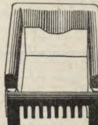
Cut Showing Arrangement of Waterbacks, Brick and Front Grates in Fire Box of Range
