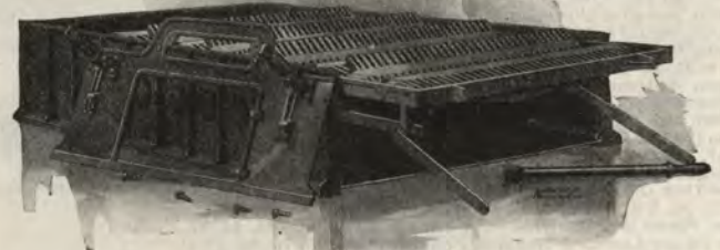
Showing Grate Frame drawn out to Repair Grates.
