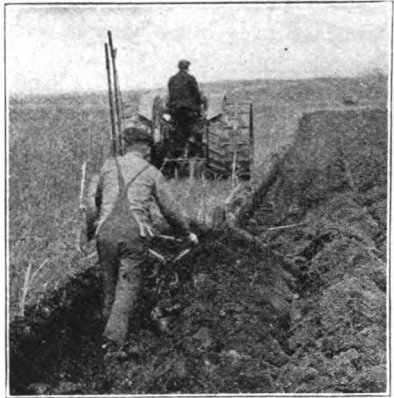
Illust. 55. Three sets of rear wheel extensions needed for this marsh land.
