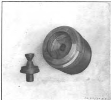
Fig. 22. The Hub and Finished Face of the Pattern
