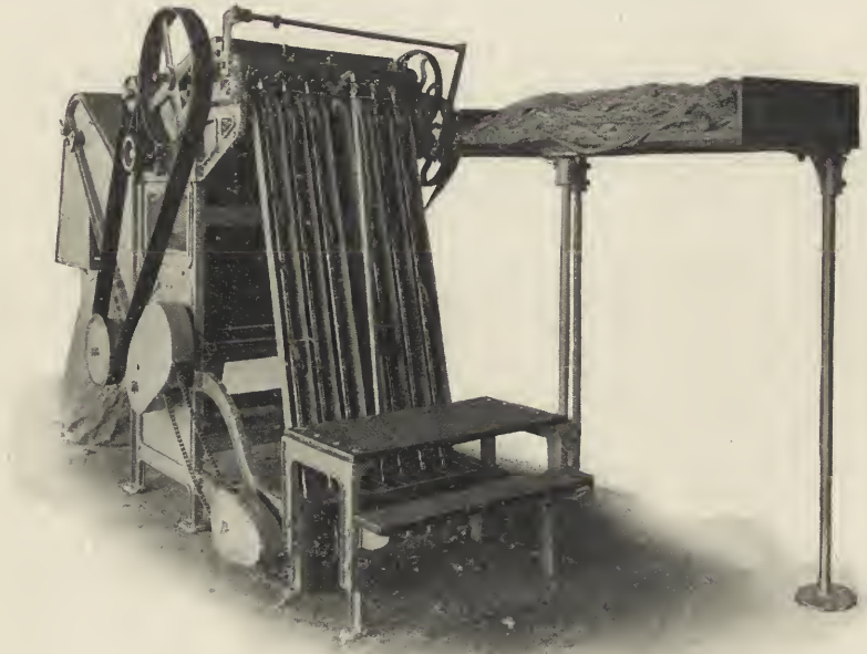
FIG. 71.—Eves' patent rope untwister and opener, as supplied by Mr W. Carter, 28 Waring Street, Belfast.
