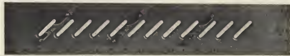
FIG. 41.—Patent conductor on under side of sliver plate. (As supplied by Messrs James Mackie & Sons, Ltd., Belfast.)
