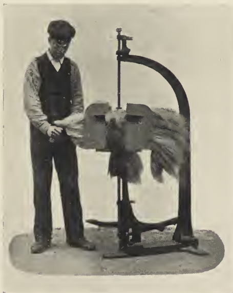
FIG. 12.—Ordinary tipping for hackler. (Apparatus supplied by W. Carter, 28 Waring Street, Belfast.)
